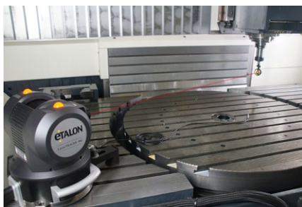
Complete measurement of linear machine tool axes
