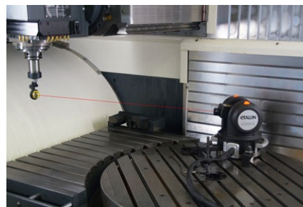
Complete measurement of rotary table axis of a machine tool
